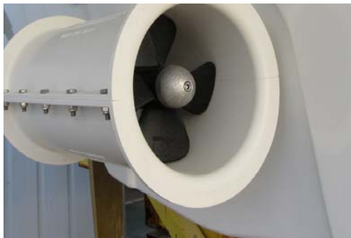
Poop thruster anode
