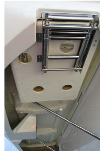
Configuration of reboarding device in the event of an accidental fall: (Ref 1)
