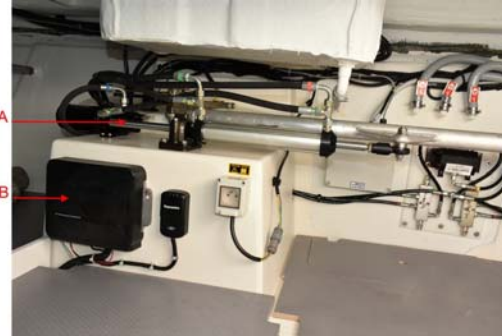
A. Hydraulic piston B. Vessel Management Unit
