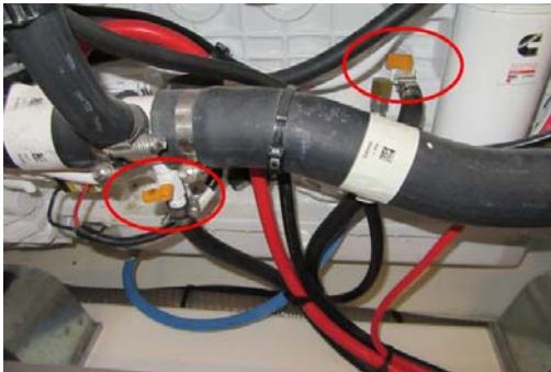
Starboard engine / water heater cooling circuit supply valve
