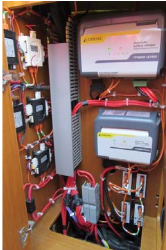
Stern thruster battery charger (24V circuit)
