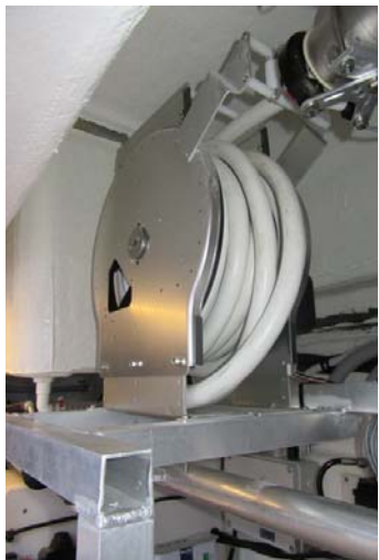
Roller for shore power lead Location: Cockpit locker
