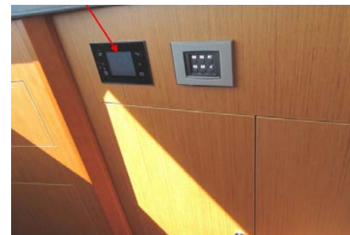
Blackwater tank gauge & Masher control Location: Touch screen
