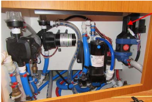
Collector drainage pump to the sea Location: Companionway
