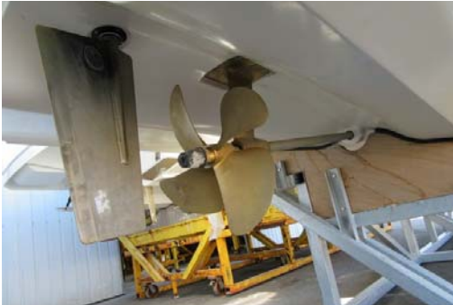
Installation of shaft engine with bracket
