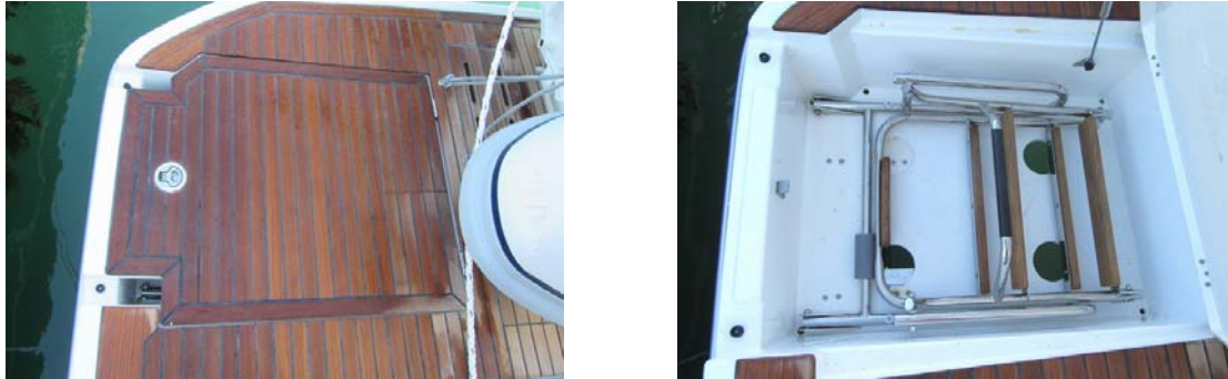
Configuration of reboarding device in the event of an accidental fall: (Ref 1)
