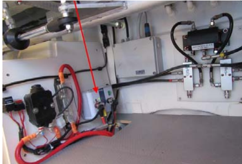
Stern thruster battery charger (24V circuit)
