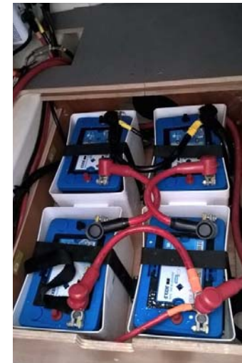
Poop thruster battery: 4 x 50A (24V circuit) Location: Cockpit locker
