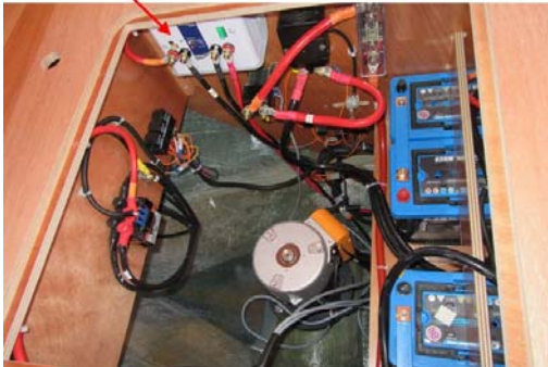
Bow thruster battery charger (24V circuit)
